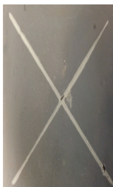
Figure 3. Aspect of coated samples (100mm by 150mm - 4 by 6 in.) before salt spray test
