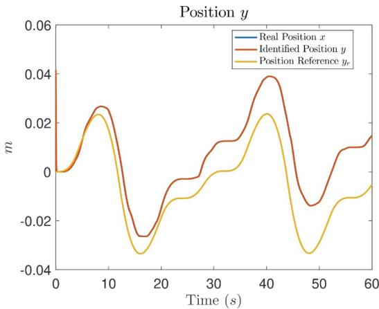
Figure 19. Comparative graph between the measured real position  $y$ , the identified  $\hat{y}$  and reference  $y_r$  of Test 3
