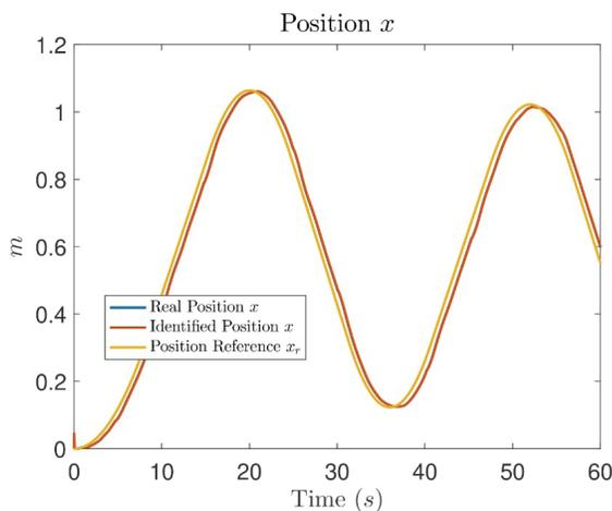
Figure 12. Comparative graph between the measured real position  $x$ , the identified  $\hat{x}$  and reference  $x_r$  of Test 2
