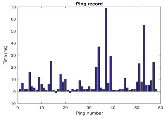
Figure 17. Ping record of Test 3. Ping statistics: Packets: Sent = 58, Received = 56, Lost = 2 (3 % Loss). Approximate round trip in milliseconds: Minimum = 1 ms, Maximum = 69 ms, Media = 8 ms
