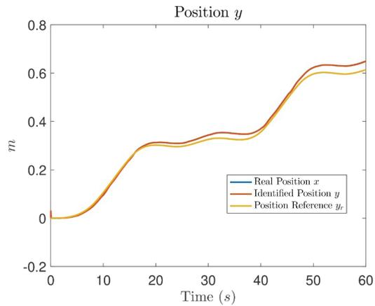
Figure 13. Comparative graph between the measured real position  $y$ , the identified  $\hat{y}$  and reference  $y_r$  of Test 2
