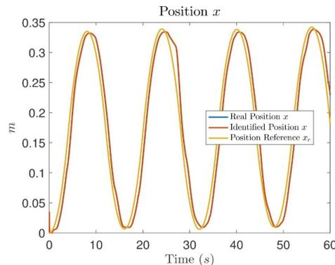
Figure 18. Comparative graph between the measured real position  $x$ , the identified  $\hat{x}$  and reference  $x_r$  of Test 3
