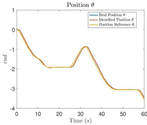
Figure 7. Comparative graph between the measured real position  $\theta$ , the identified  $\hat{\theta}$  and reference  $\theta_d$  of Test 1
