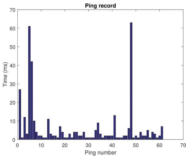
Figure 11. Ping record of Test 2. Ping statistics: Packets: Sent = 61, Received = 61, Lost = 0 (0 % Loss). Approximate round trip in milliseconds: Minimum = 1 ms, Maximum = 63 ms, Media = 6 ms
