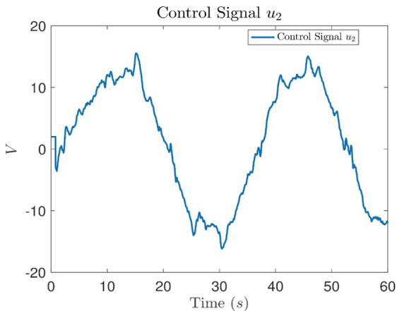
Figure 16. Control signal  $u_2$  of Test 2
