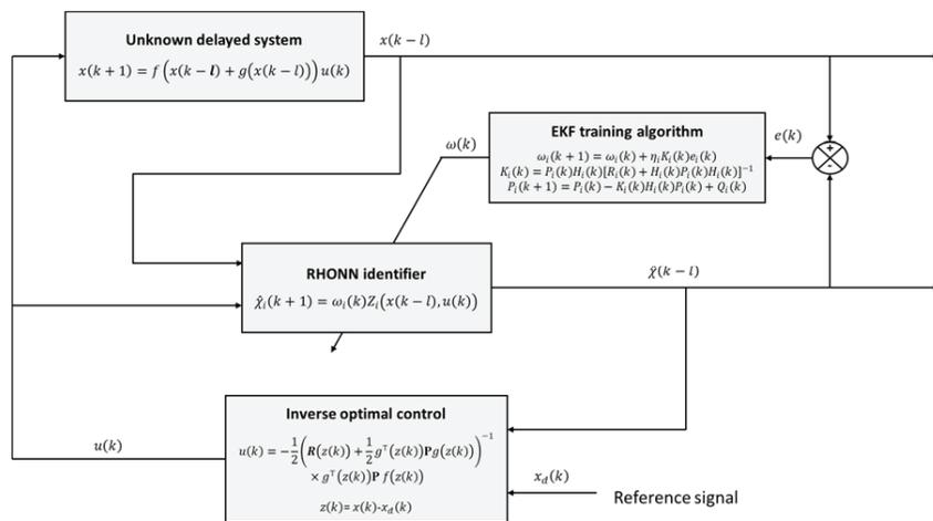
Figure 1. Neural inverse optimal control scheme
