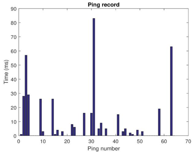
Figure 4. Ping record of Test 1. Ping statistics: Packets: Sent = 64, Received = 64, Lost = 0 (0 % Loss). Approximate round trip in milliseconds: Minimum = 0 ms, Maximum = 83 ms, Media = 6 ms. Please note that in the graphic values of zero represent results of less than 1 ms
