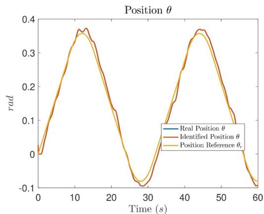
Figure 14. Comparative graph between the measured real position  $\theta$ , the identified  $\hat{\theta}$  and reference  $\theta_r$  of Test 2
