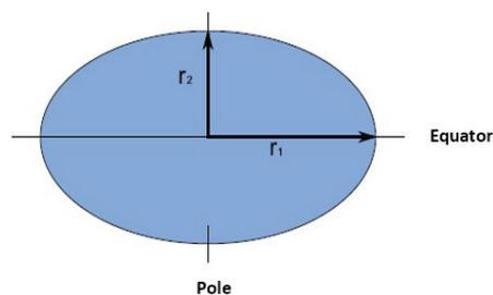
Figure 5. Reference ellipsoid. Adapted from (Olaya, 2014)
