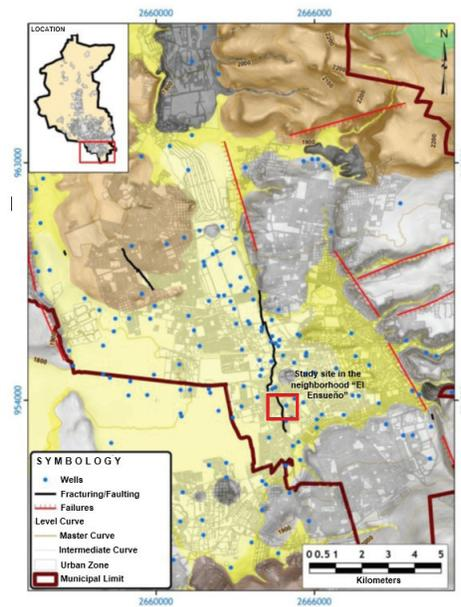
Figure 3. Fault system in the Central Zone and location in the "El Ensueño" (Protección Civil, 2015)
