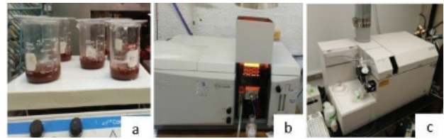
Figure 6. a) Leaching process, b) atomic absorption equipment, c) HPL equipment used
