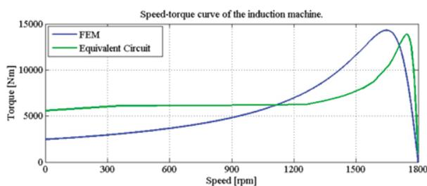
Figure 14. Speed-torque curve
