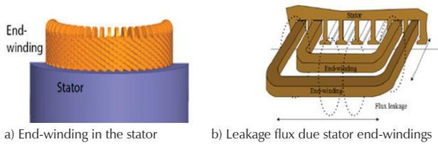
a) End-winding in the stator b) Leakage flux due stator end-windings
