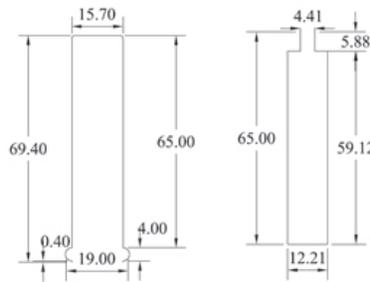
Figure 9. Stator and rotor slots dimensions (mm)
