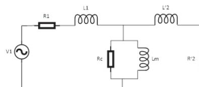
Figure 1. Single-phase equivalent circuit (referred to the stator) of a balanced three-phase squirrel cage motor
