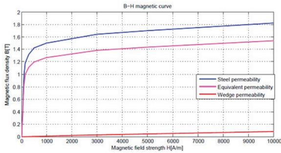
Figure 4. B-H curve of the motor magnetic materials
