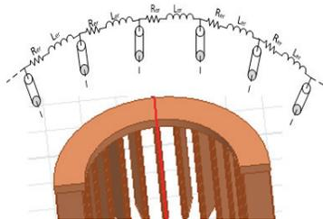
Figure 6. Equivalent circuits representing the squirrel-cage
