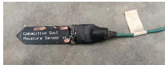
Figure 9. Sensor surface wearing
