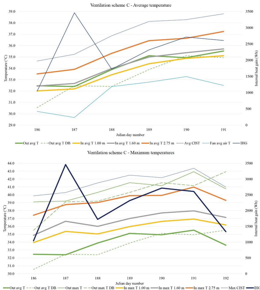
Figure 8. Daily average and maximum temperatures of the monitoring period with ventilation scheme C
