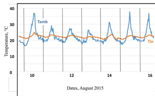
Figure 8a. Interior temperature (Tin) v ambient temperature in Summer
