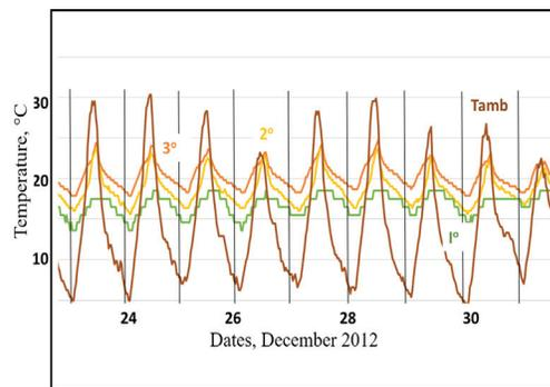
Figure 9. Temperatures in floors 1, 2 and 3 v ambient temperature
