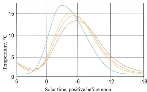
Figure 13. Ambient temperature variation (blue) gets damped with increased atrium height
