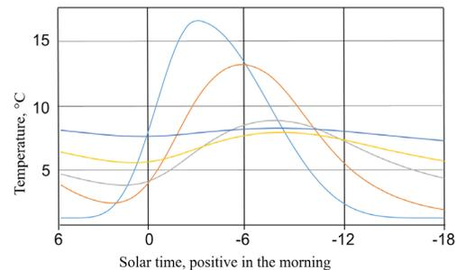
Figure 15. Air temperature variation is damped with atrium blocking
