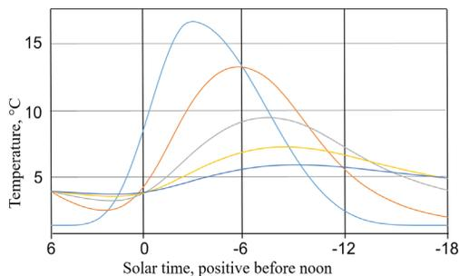
Figure 14. Air temperature variation (blue) is damped with building mass
