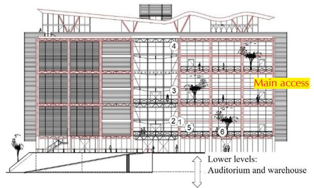
Figure 2. Office building block and location of thermal sensors
