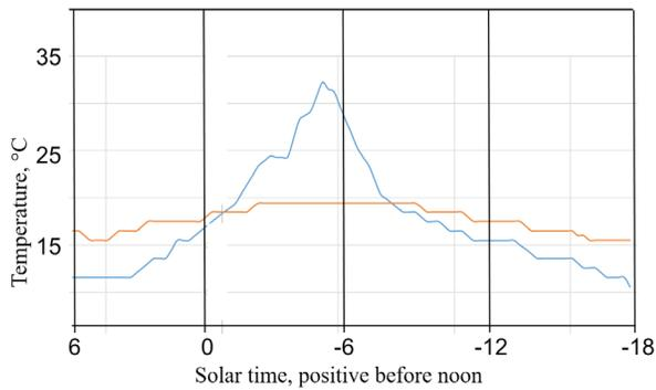
Figure 12a. Typical temperature measurements for ambient (blue) and inside (orange)
