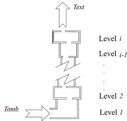
Figure 11. Simplified air flow diagram for  $i$  building levels
