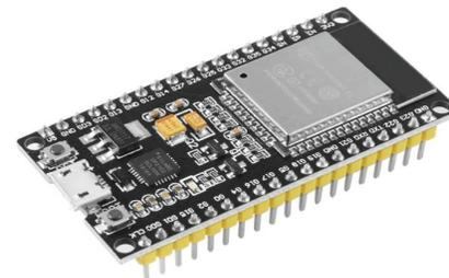
Figura 5. ESP32 NodeMCU-32 BT+WiFi 38 Pines, (TresD Print Tech, 2023).
