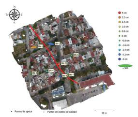
Figure 15. Location of each GCP and error estimation using Agisoft MetaShape software
