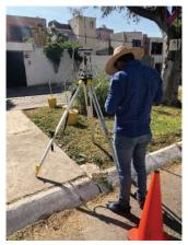
Figure 10. GCP measurement in the "El Ensueño" with the Sokkia GRX2 GPS
