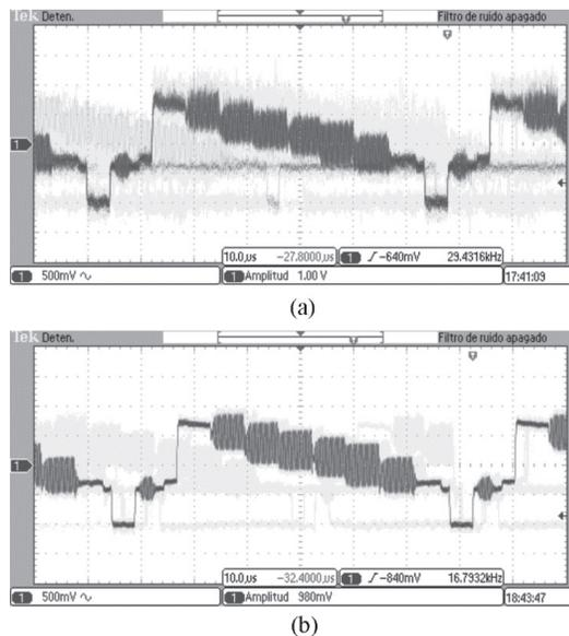
Figure 9. Photoreceived analog video, on depending on the received optical power 2.5W: a) PIN photodetection of 2.5  $\mu$ W, b) APD photodetection of 0.25  $\mu$ W
