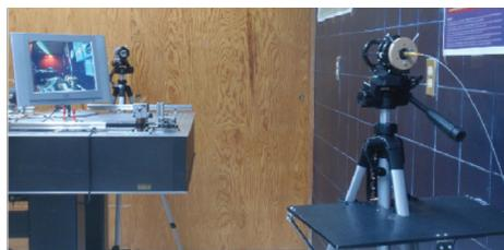
Figure 10. Experimental FSO link when transmitting a live NTSC video signal
