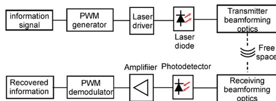
Figure 1. The proposed free-space optical link based on PWM
