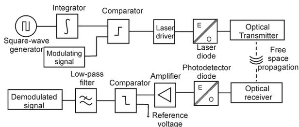
Figure 3. Free-space optical link base on PWM subcarrier
