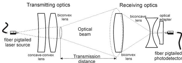
Figure 2. The free-space optics transmitter and receiver subsystems
