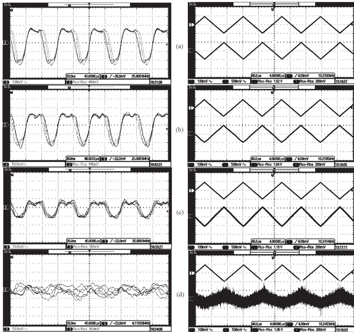
Figure 6. Photodetected signal waveforms corresponding to received optical power based on PIN photodetector: a)  $10 \mu\text{W}$ , b)  $5 \mu\text{W}$ , c)  $2.5 \mu\text{W}$ , d)  $1 \mu\text{W}$
