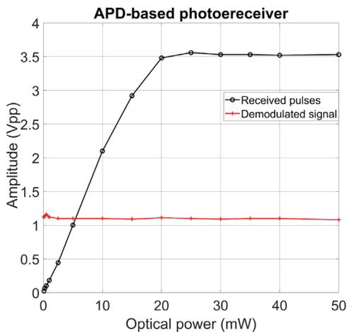
Figure 7. Photodetection based on APD photodetector, black-dots trace corresponds to received optical pulses, red-crosses trace shows the demodulated signal amplitude
