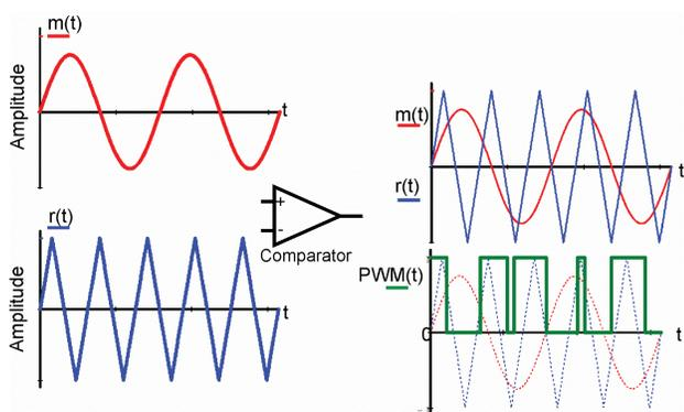
Figure 4. PWM signal generation for free-space optical transmission
