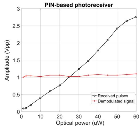
Figure 5. Photodetection based on PIN photodetector, black-dots trace corresponds to received optical pulses, red-cross trace shows the demodulated signal amplitude
