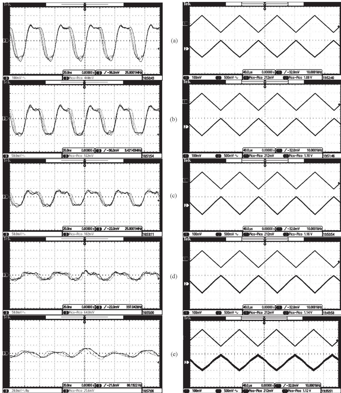
Figure 8. Photodetected signal waveforms corresponding to received optical power based on APD photodetector: a) 2.5  $\mu\text{W}$ , b) 1  $\mu\text{W}$ , c) 0.5  $\mu\text{W}$ , d) 0.25  $\mu\text{W}$ , e) 0.1  $\mu\text{W}$
